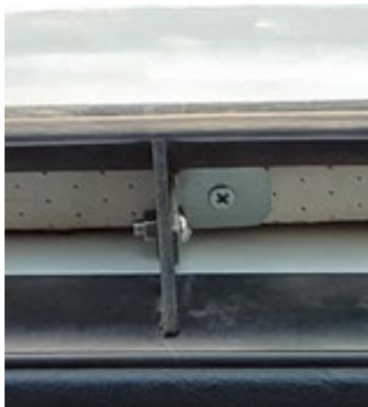
Insertion rubber placed between stiffeners and car body.
