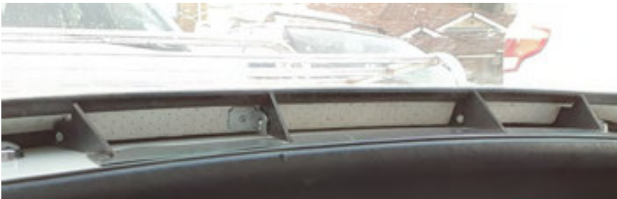
View of four stiffeners spaced out for maximum effect.
